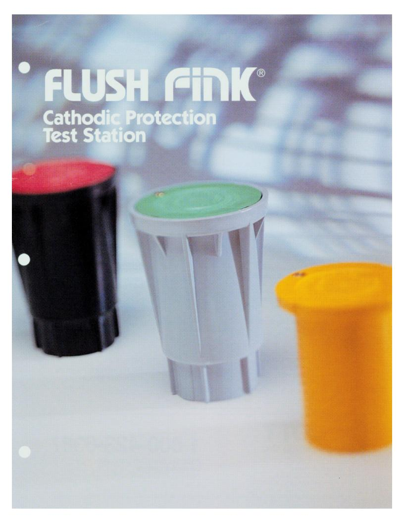
The **FLUSH** cathodic protection test station and terminal enclosure is a high strength, maintenance free, non-conductive, flush mounted below ground terminal. It's patented "Bell Jar" design keeps test leads dry even when the enclosure is covered by flood water. Field proven since 1978, **FLUSH** FINK® is manufactured by Cott in Pittsburgh, Pennsylvania and Los Angeles, California. It is available from Cott distributors everywhere.
